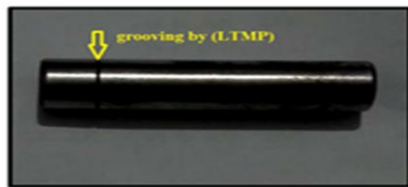
(a) photo of single grooved specimen
