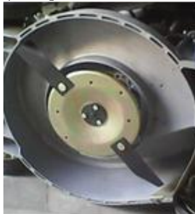
Fig. 6: Photograph of cutting knives of imported grass-mower.
