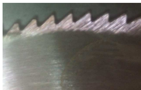
Modified saw disc (100 teeth with sharp edge)
