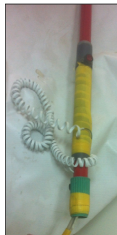
B. An image of telescopic picking hand stick equipped with swing type push on/off switch.
