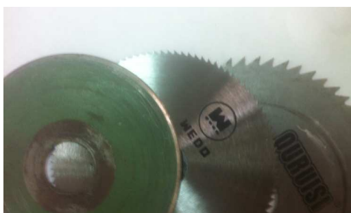
Plan discs, 100 teeth discs, and 50 teeth discs
