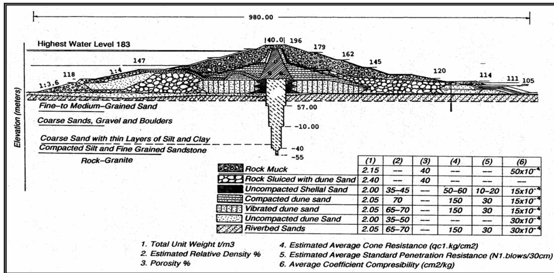
Fig. 1 The Aswan High Dam Cross section, Abdel Azim Abul-Atta, [1]
