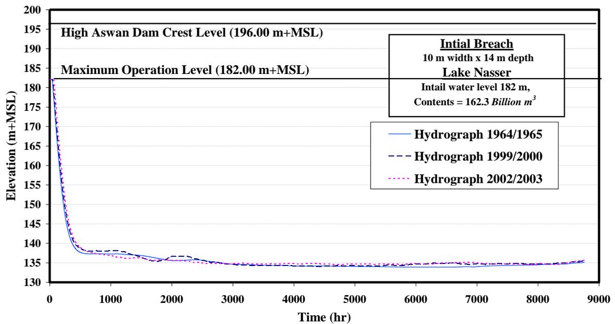
Fig. 10 Water level of the Nasser Lake for scenarios No. 1, 2, and 3
