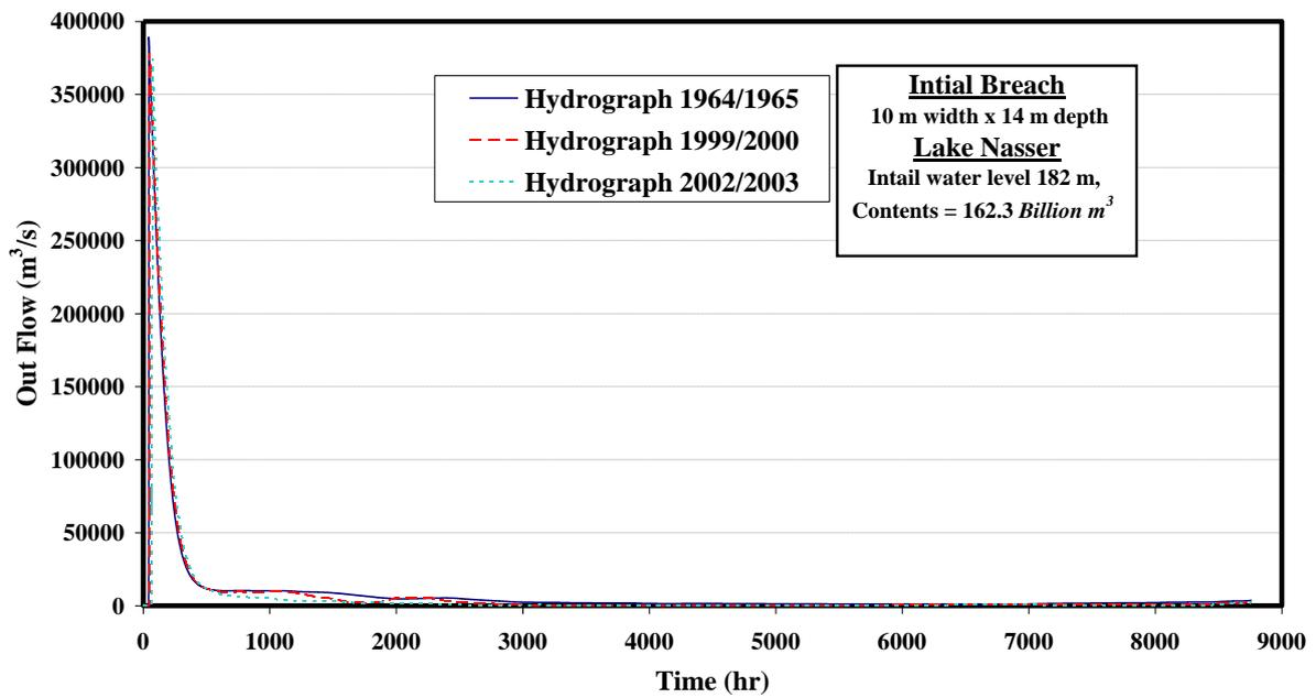
Fig. 9 Outflow hydrograph of scenarios No. 1, 2, and 3
