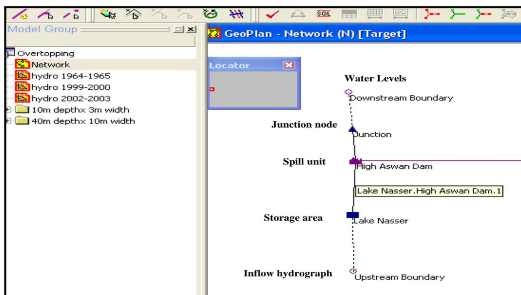
Fig. 6 The network at the HR BREACH model
