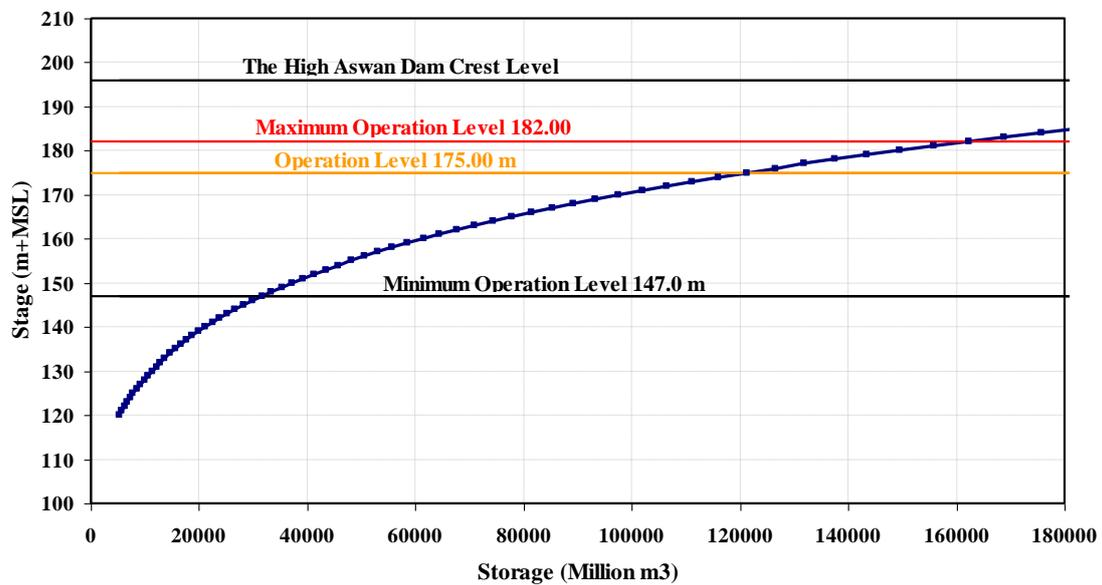
Fig. 2 Nasser Lake Elevation-storage curve
