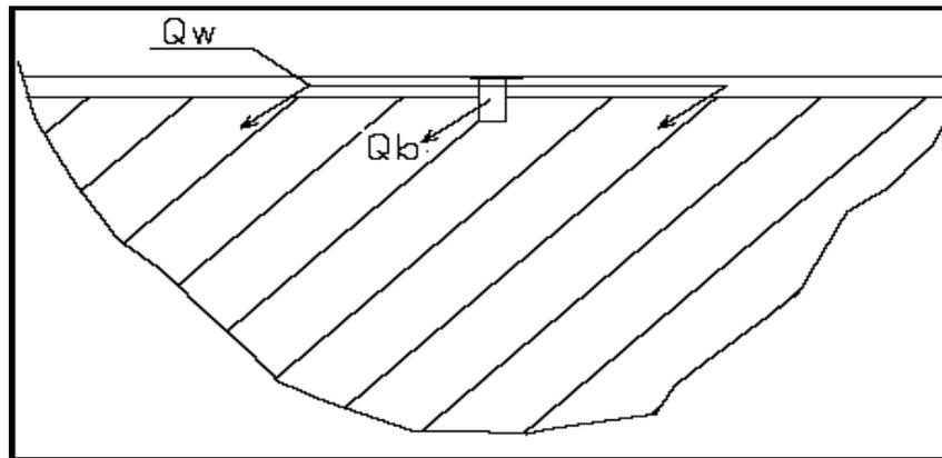
Fig. 4 Flow computations through the breach and over the dam, M. A. Mohamed, and et. al [5]
