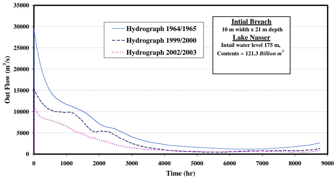
Fig. 11 Outflow hydrograph of scenarios No. 4, 5, and 6
