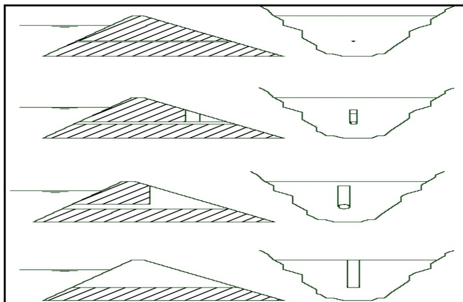
Fig. 5 Mechanism of piping failure, M. A. Mohamed, and et. al [5]
