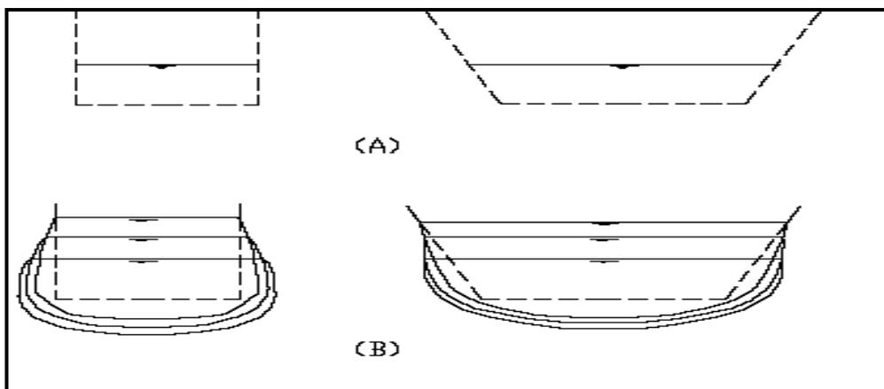
Fig. 3 a. initial breach shape
