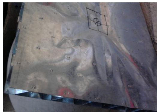
Fig. 21 Experimental mode of failure for TCP panel tested
