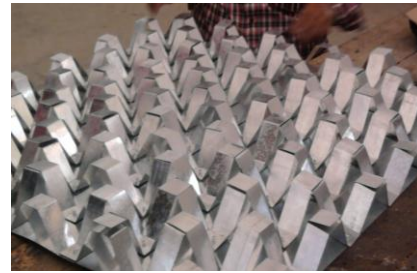
Fig. 7 Manufacturing process of corrugated core
