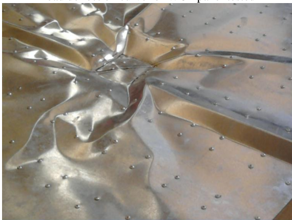
Fig. 17 Experimental mode of failure for WCP panel tested
