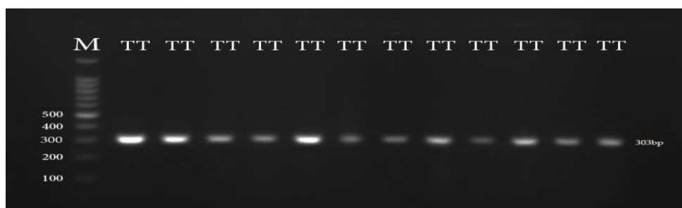
Figure 1: Ethidium bromide stained 2% agarose gel electrophoresis of representative samples of RFLP banding pattern of LHR gene (part of exon 11-303 bp) from normal fertile and repeat breeder buffaloes after digestion with HhaI . M: 100 bp ladder.
