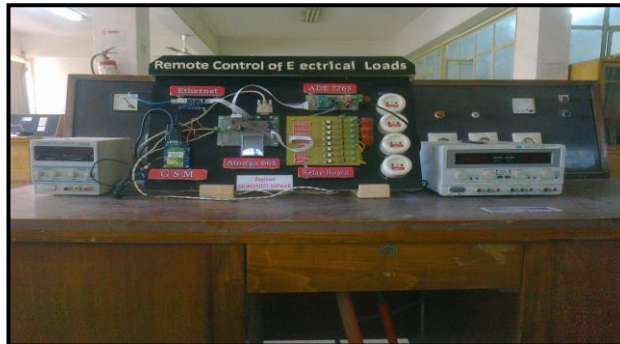
Fig 9 : The photo of the electronic device during measurements.
