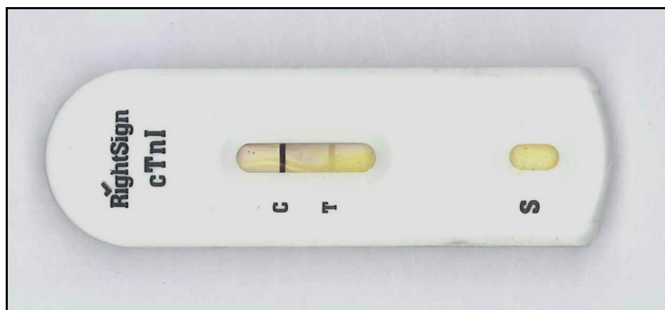
Photo 3. Rapid cTnI assay kit, weak positive in serum, 1 non clear (light) red brown line appears in the test line region parallel to the control line
