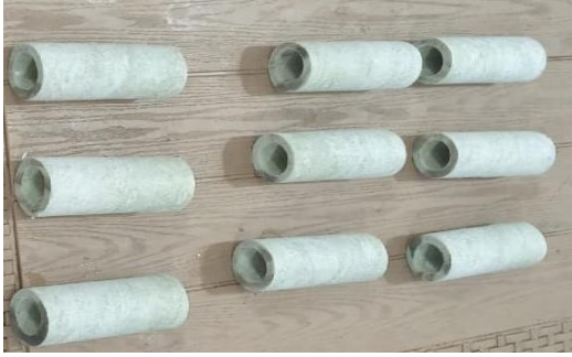
Figure 2- A photograph of the prepared GFRP specimen tubes cut from the initial filament wound tubes to be externally turned.
