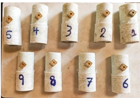
Figure 5- A photograph of GFRP tubes after turning along with their own fresh insert turning tools.
