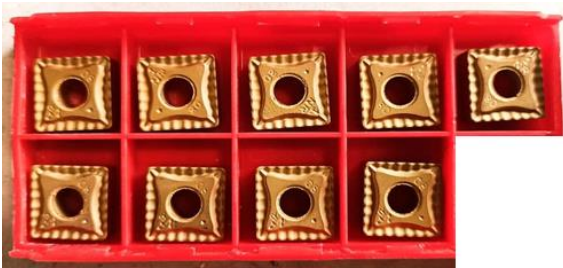
Figure 4- Nine fresh HSS insert turning tools used for turning tests.
