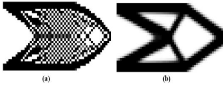
Fig. 9. Difference between topological design (a) without mesh filtering and C= 64.6405 . (b) with mesh filter and C= 66.6591 .
