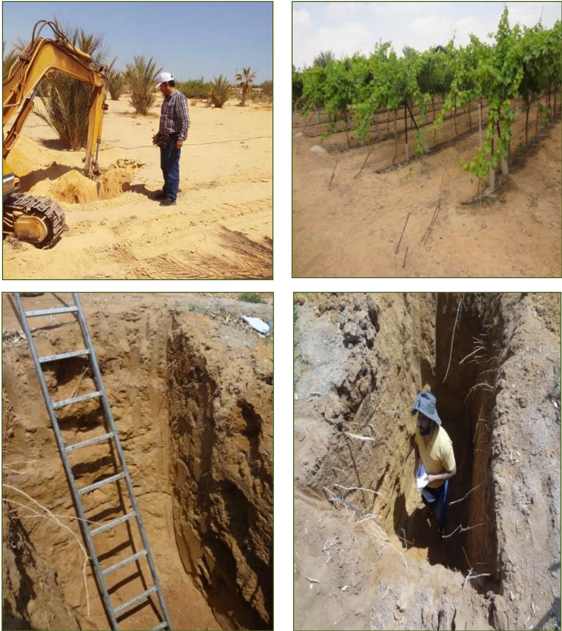
Fig. 6. A broad excavation across the research area offers for pedon description activities.
