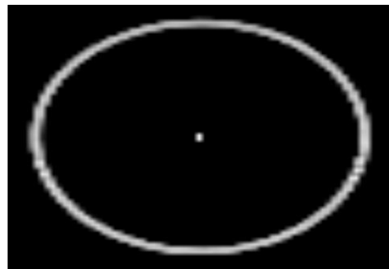
Figure (3) CT image of a thin tungsten wire used to calculate MTF.
